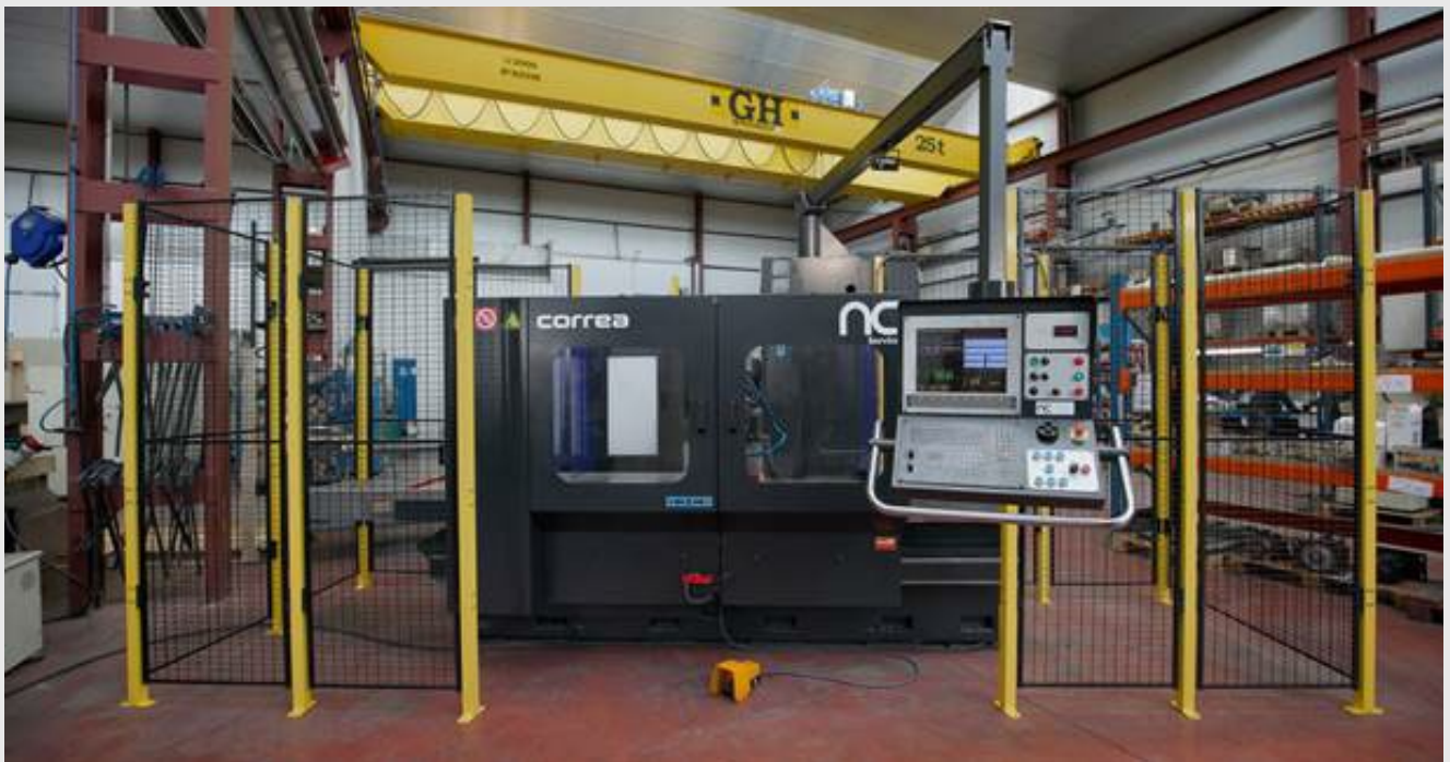
CORREA CF 17D milling machine after full mechanical retrofitting process
