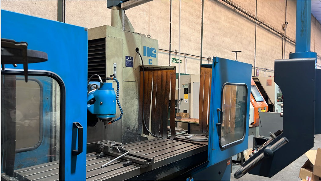
CORREA CF 17D milling machine at origin, before retrofitting process
