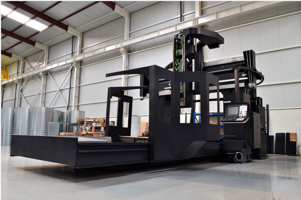
CORREA FP 40/40 milling machine during its retrofitting process
