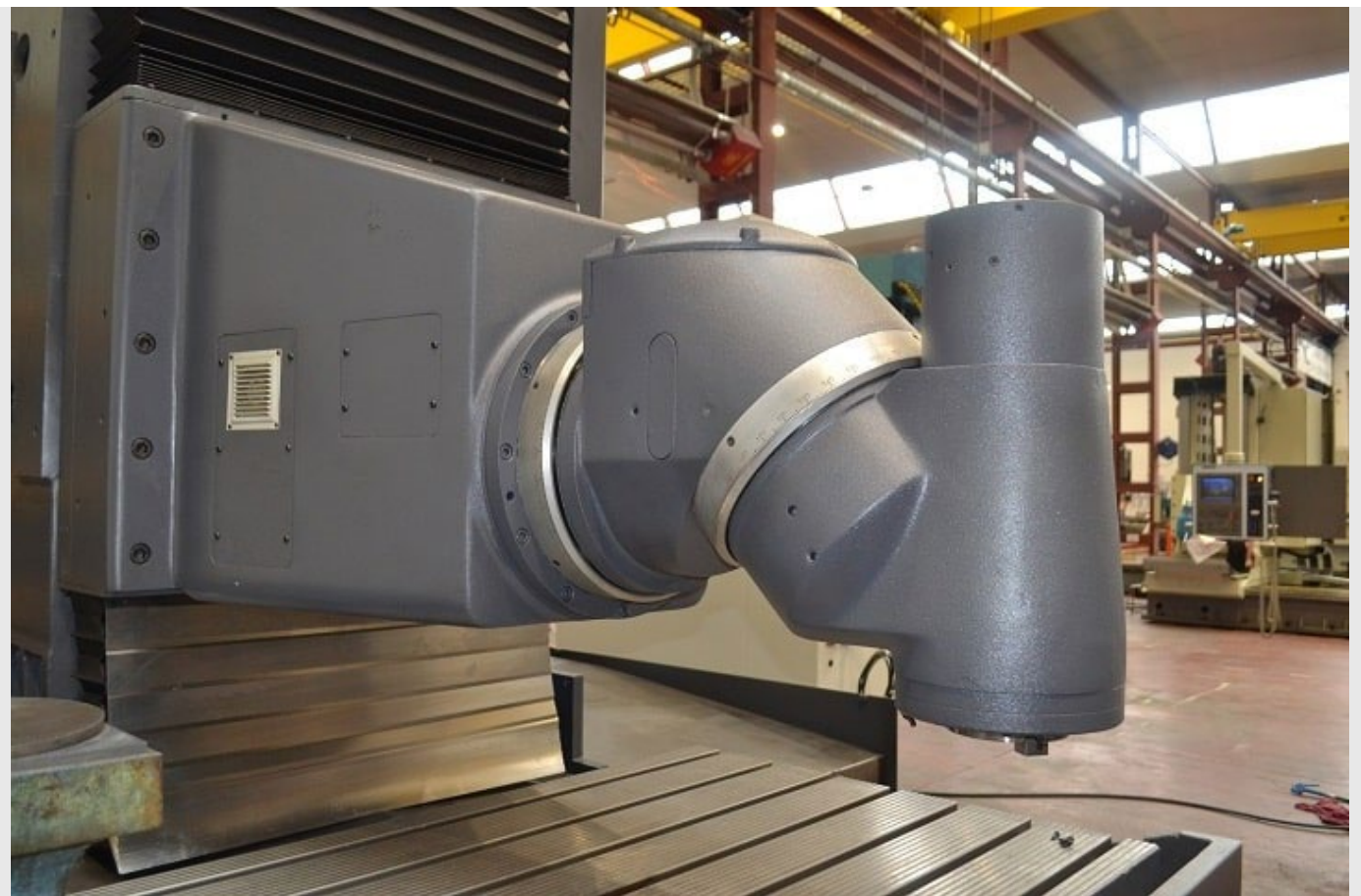
Detail of BIRA head during refurbishment of ANAYAK HVM 3300 milling machine
