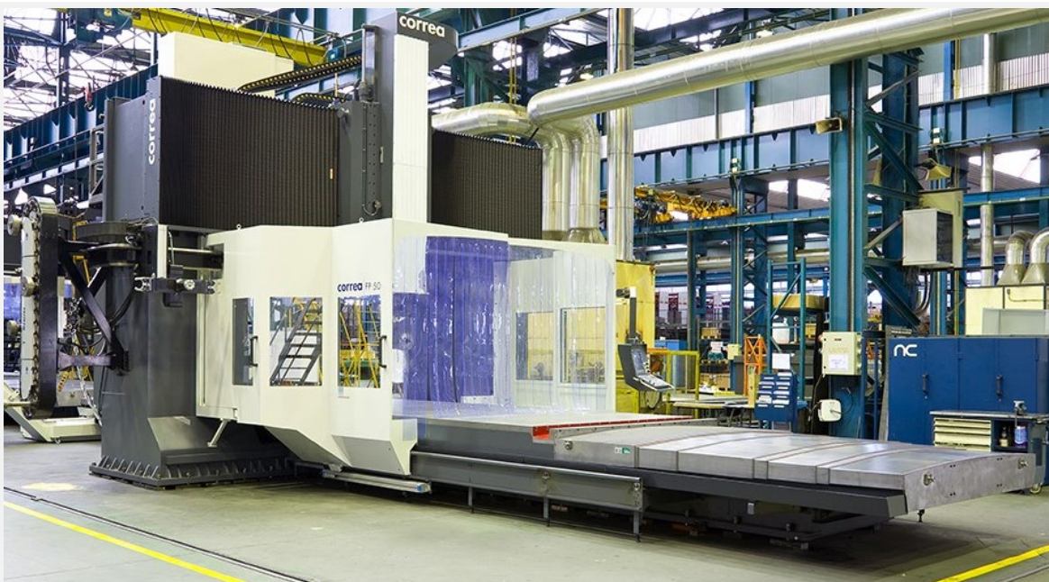
Example of a CORREA FP 50/50 milling machine after retrofitting process with ATC option
