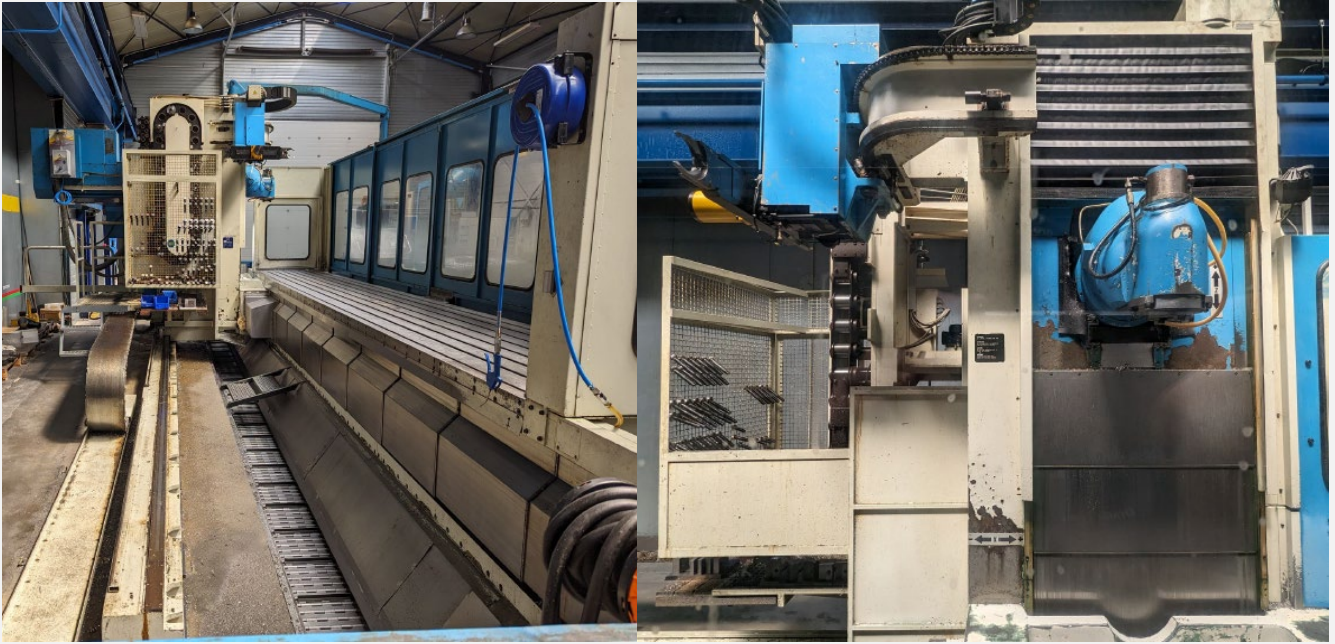
CORREA L30/58 milling machine before refurbishment (in origin)
