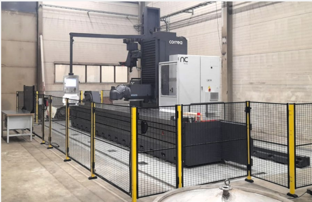
Example of a CORREA L30/58 milling machine after full retrofitting with new TNC
